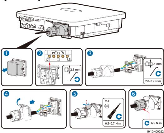
Figure 5-5 Securing the AC connector
