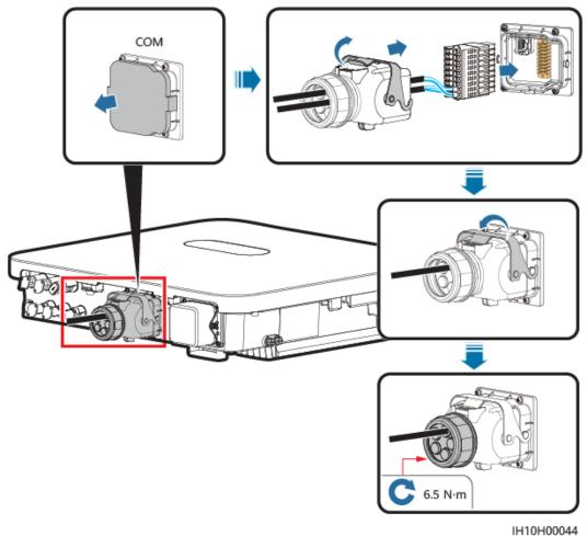
Figure 5-40 Securing the signal cable connector
