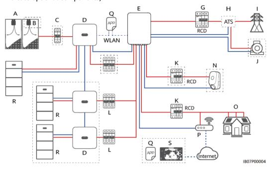
**Figure 2-5** Networking with some of loads connected to the SmartGuard (dashed boxes indicate optional components)
