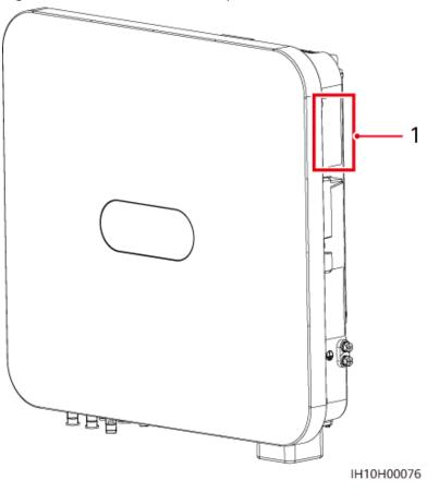
Figure 2-9 Position of the nameplate
