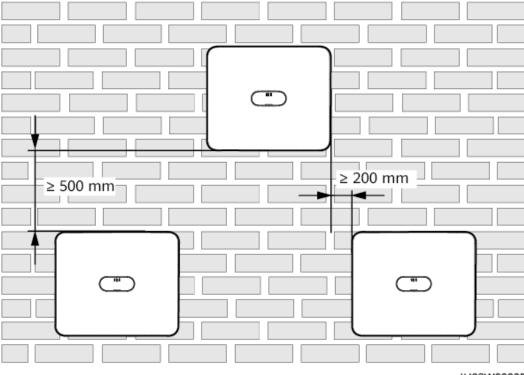
Figure 4-4 Triangle installation mode (recommended)
