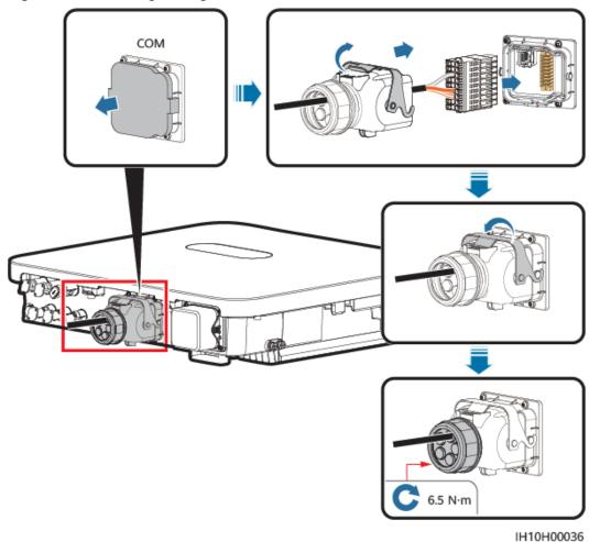
Figure 5-27 Securing the signal cable connector
