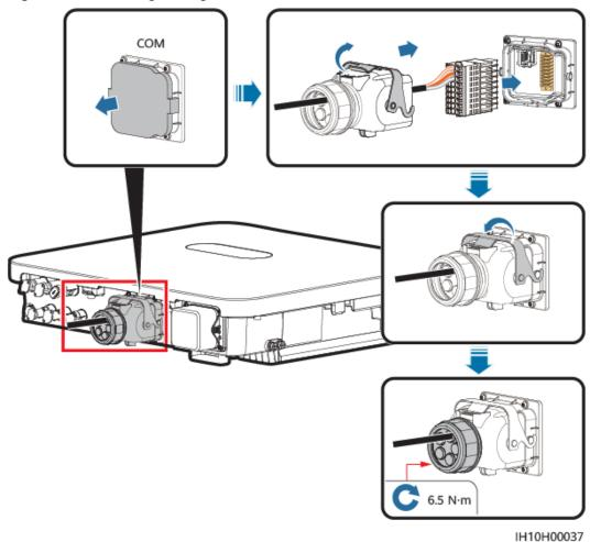
Figure 5-29 Securing the signal cable connector
