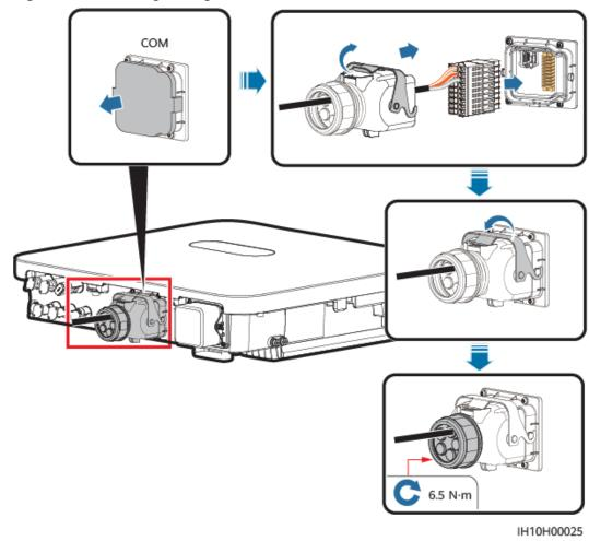
Figure 5-20 Securing the signal cable connector
