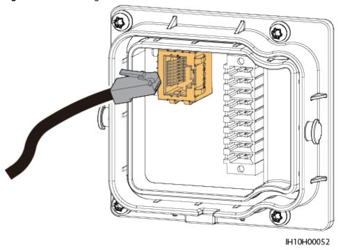
Figure 5-42 Installing the cable
