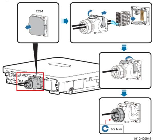
Figure 5-34 Securing the signal cable connector
