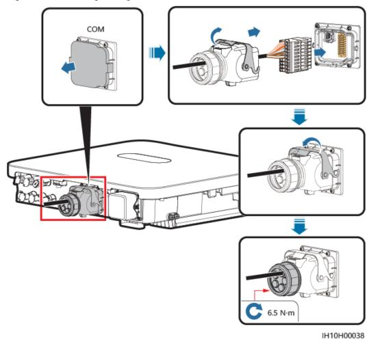
Figure 5-31 Securing the signal cable connector
