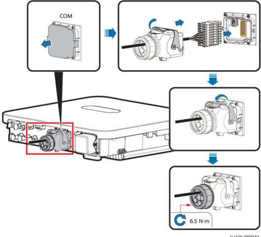
Figure 5-37 Securing the signal cable connector
